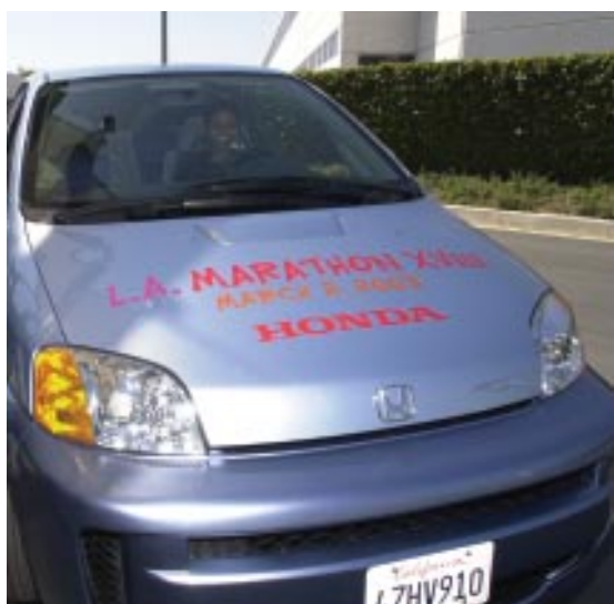
The Honda FCX, left, is a zero-emission four-seater with a 220-mile range; this one was the pace car in the recent L.A. Marathon. It's pretty standard inside, above, but there's a sleek electric motor under the hood (the fuel cell sits under the middle of the body), and the fill pipe looks different, right.
